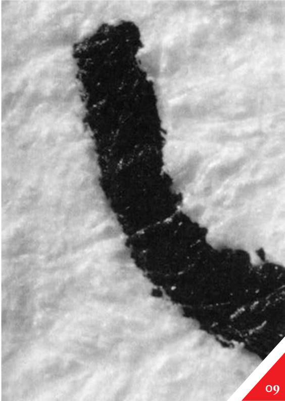
Figure 9: Paper with typed text onto Strathmore 20% cotton fiber typewriter stock with text applied by a Brother Ax-22 electronic typewriter from a Brother correctable cartridge. Source of original image, reproduced with permission: http://aic.stanford.edu/sg/bpg/annual/v111/bp11-01a.jpg
